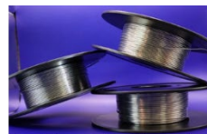
Figure 2. Copper-tin alloy metal filament with conductivities reaching 7x more resistive than bulk copper.
