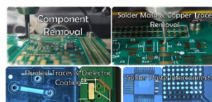
Figure 1. PCB repair steps of removing solder mask, removing components and adding conductive and dielectric for repair.
