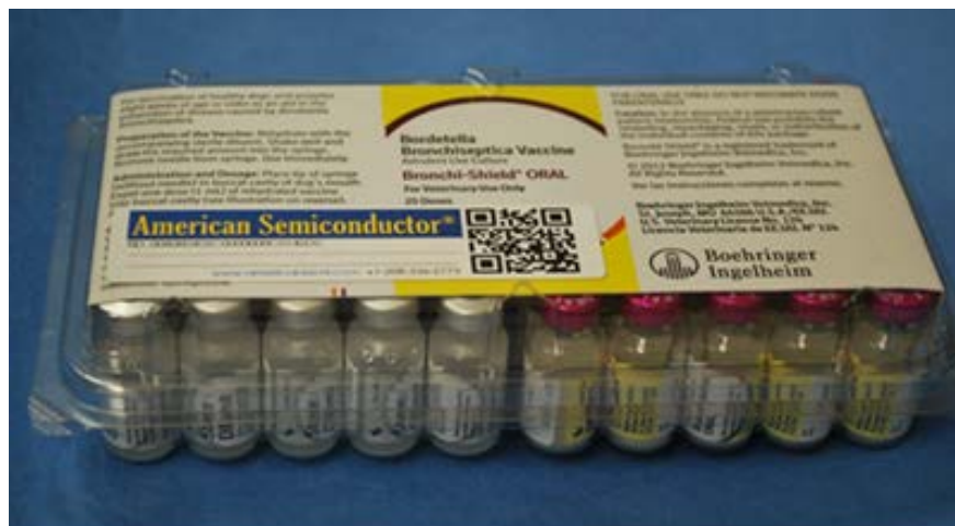
ASI GP-Tag (RF temperature sensor) mounted to the surface of a Bordetella vaccine container. This is an example of a high value product that could benefit from the Smart-Tag.
