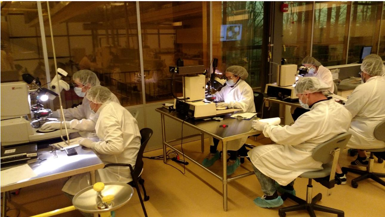
Photo: TRAIN Ohio & LCCC MicroElectronic Mechanical Systems (MEMS) students learn to use thermosonic wire bonders for wire bonding 0.001" diameter gold wire.
