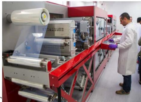
Fig 2. The multilayer, R2R processing tool at the UW's WCET with high-resolution flexography, rotary screen, offset gravure and slot die coating capability.
